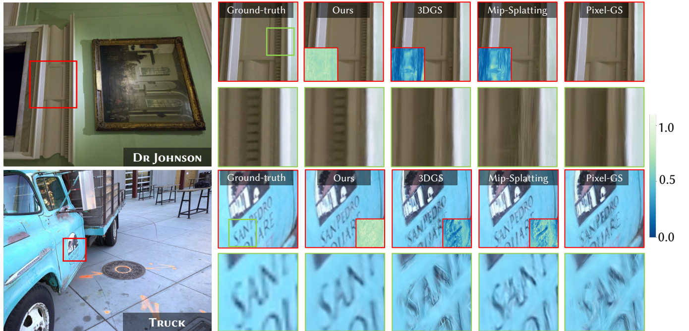
Fig. 9. Qualitative comparisons on the real scenes [Hedman et al. 2018; Knapitsch et al. 2017]. We visualize the spectral entropy maps of 3D Gaussians. Bluer regions indicate lower spectral entropy, with more needle-like degraded Gaussians, while greener regions represent higher spectral entropy.
